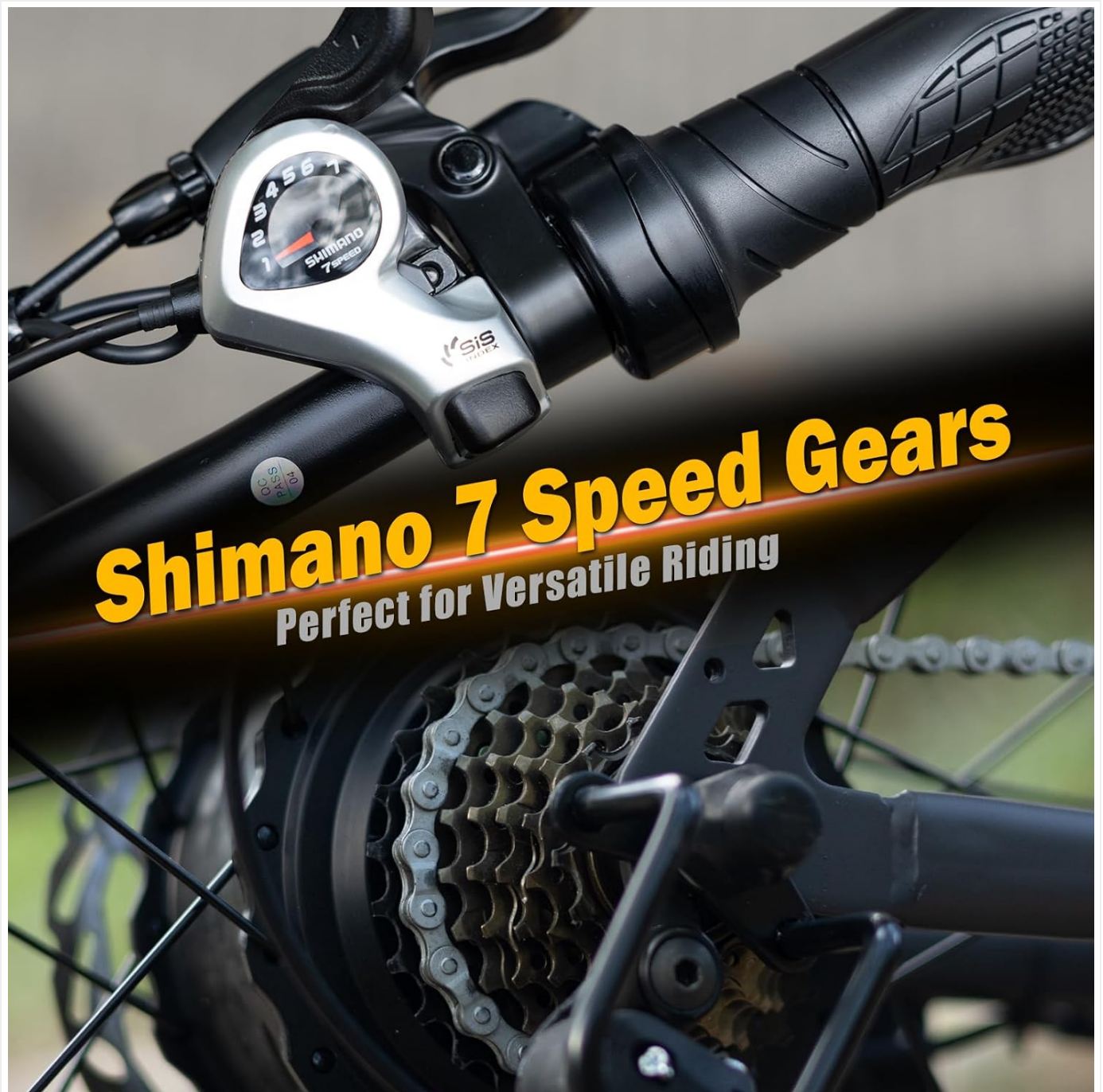
Image: Close-up of the Shimano 7-speed gear shifter and rear derailleur on the ZDZA ZA01, illustrating the gear system.
