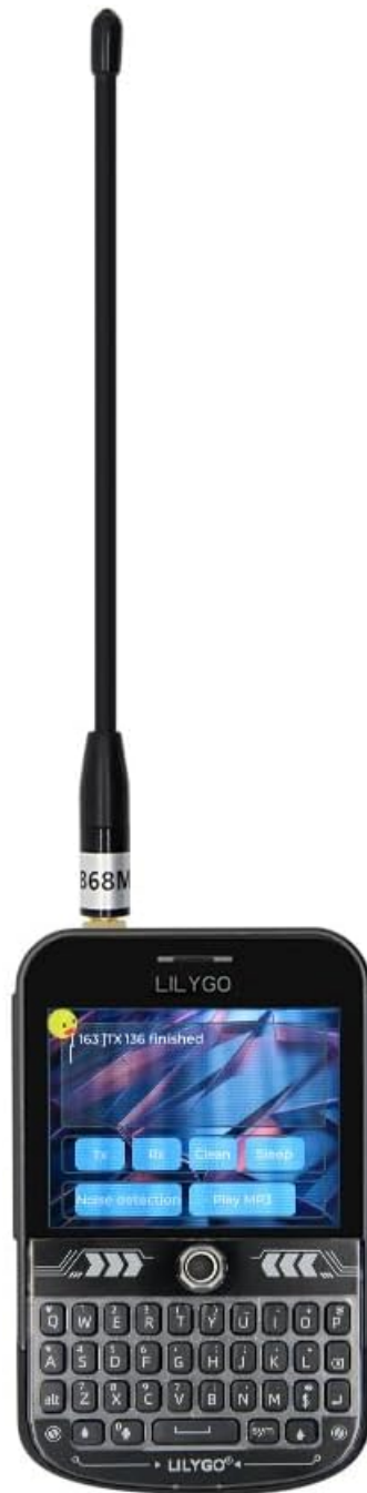
Figure 2: Front view of the LILYGO T-Deck Plus, showing the display and QWERTY keyboard.
