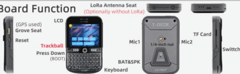
Figure 4: Detailed diagram of LILYGO T-Deck Plus features and interfaces.
