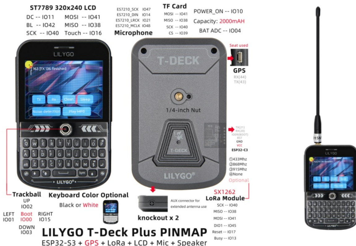
Figure 5: LILYGO T-Deck Plus pinmap and interface connections.
