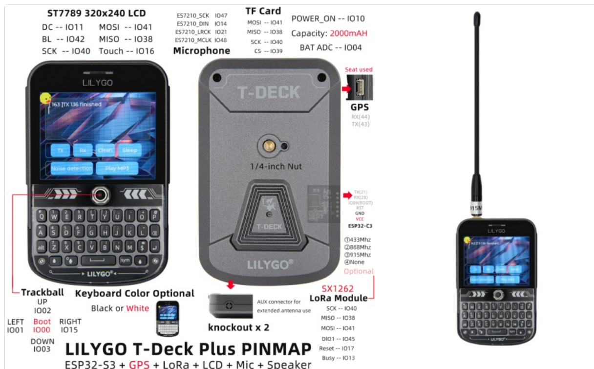
Figure 6: Detailed pinmap and component layout of the LILYGO T-Deck Plus.
