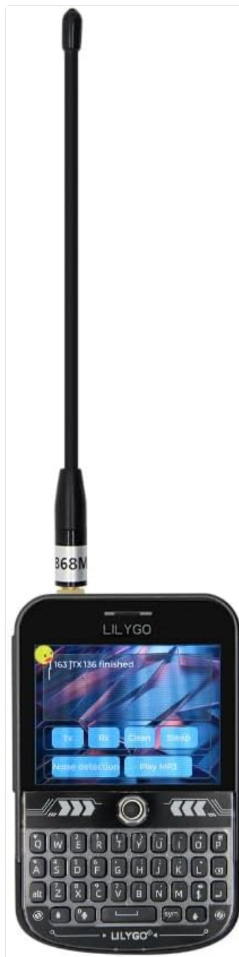
Figure 2: Front view of the LILYGO T-Deck Plus, showing the display, keyboard, and attached antenna.
