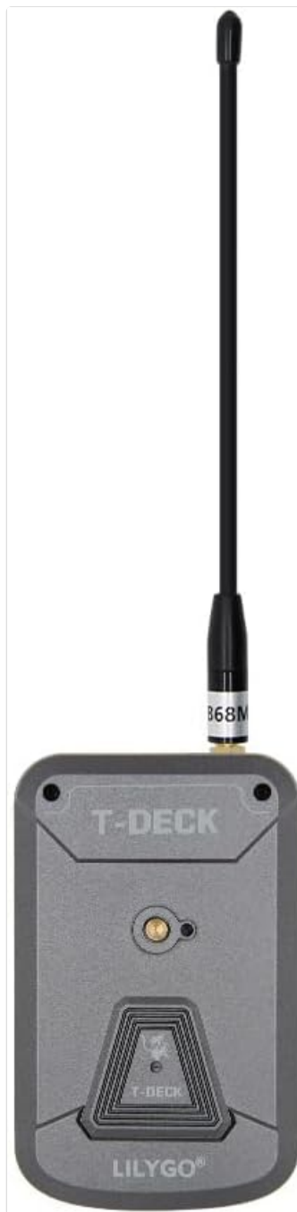
Figure 4: Rear view of the LILYGO T-Deck Plus, showing the antenna port and mounting features.
