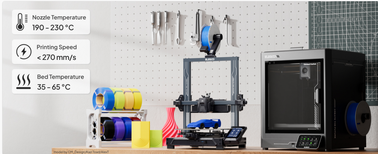
Image 3.1: Recommended printing temperatures and speed for ELEGOO PLA filament.
