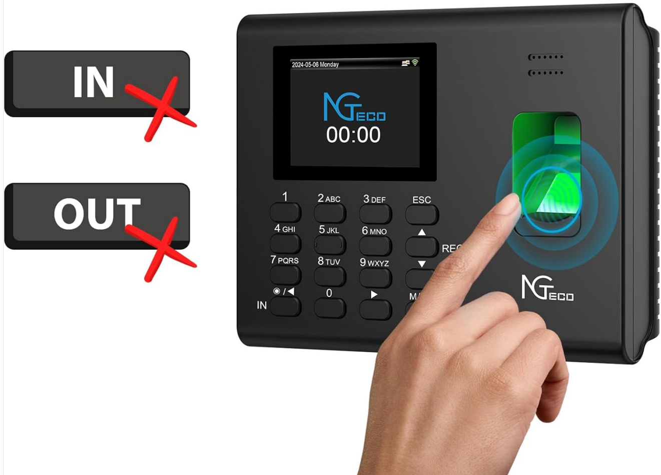
Figure 4.1: The automatic punch mode eliminates the need for manual IN/OUT key presses.
