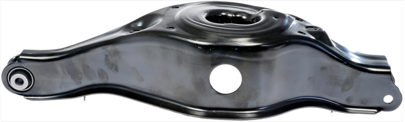
Image 7.3: Side view of the Dorman 528-101 control arm, highlighting its profile and bushing location.
