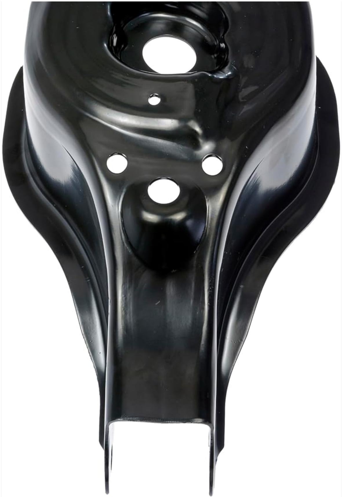
Image 7.1: Top view of the Dorman 528-101 control arm, showing mounting points and overall shape.
