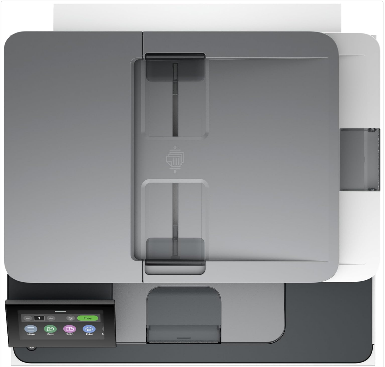
Image 5.2: Top view of the printer, illustrating the Automatic Document Feeder (ADF) for multi-page scanning and copying.
