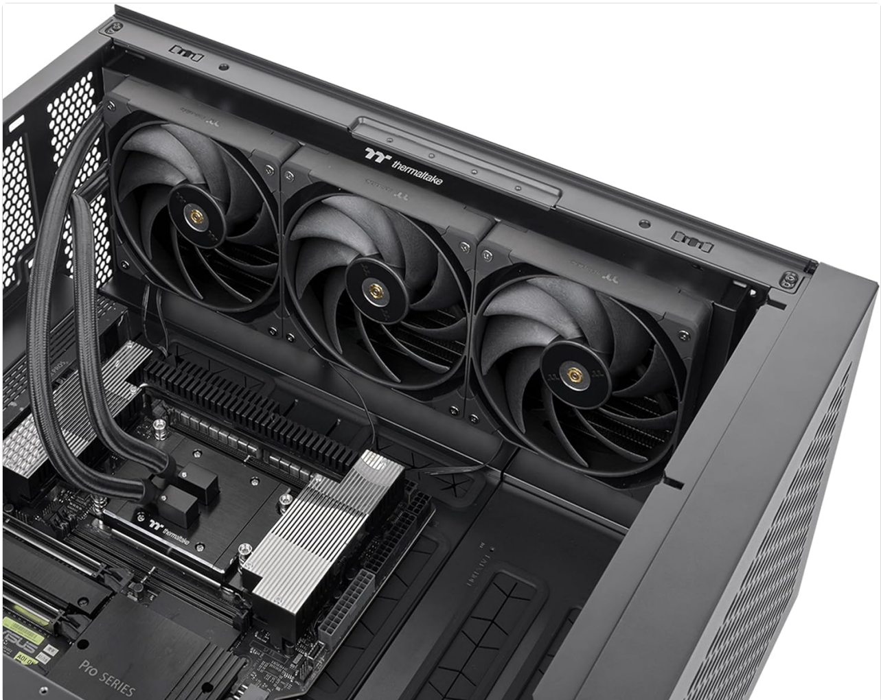
Image 4.1: AW420 Liquid Cooler installed in a typical PC case configuration.
