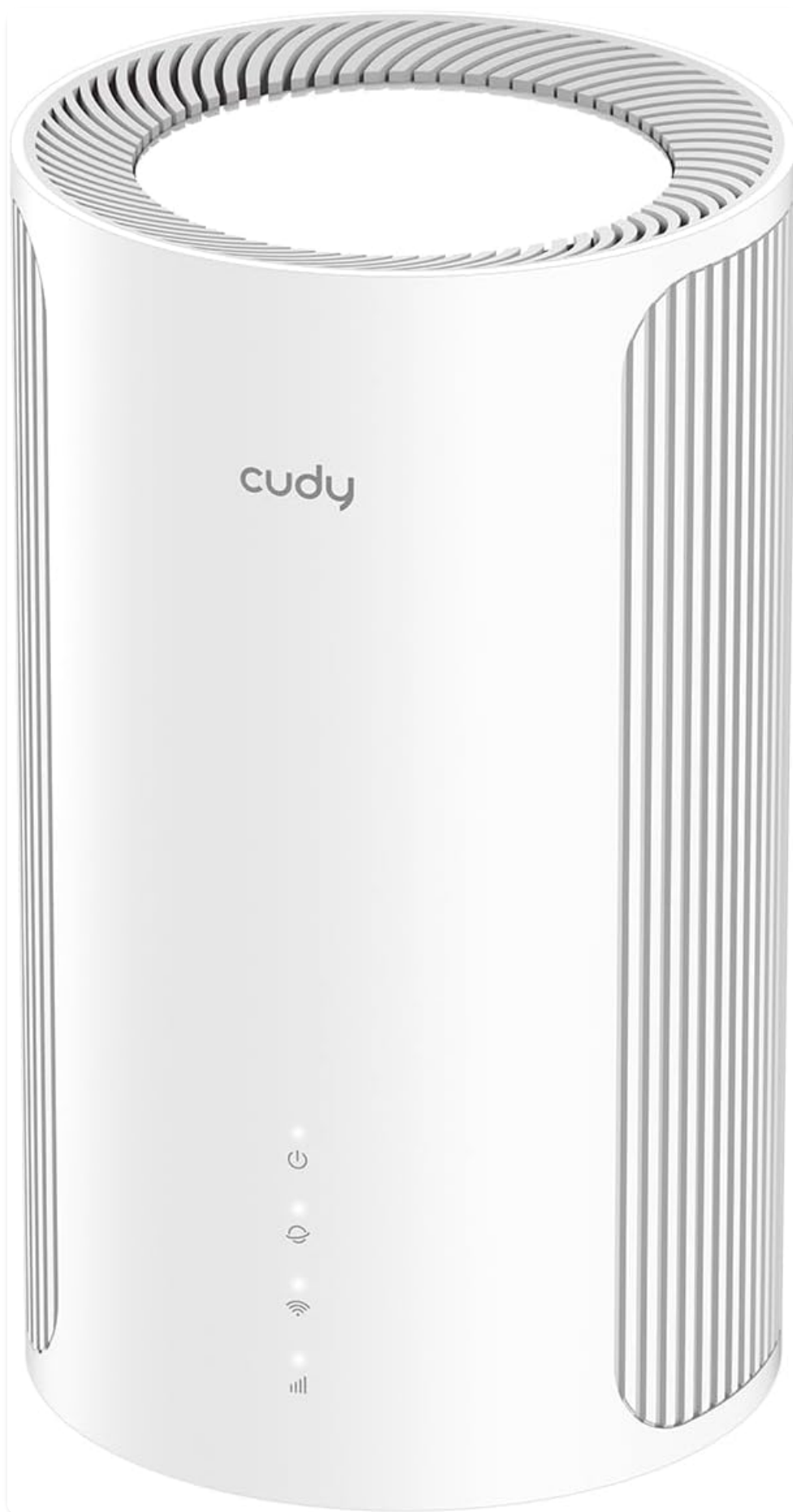
Image 1.1: The Cudy P2 AX3000 Wi-Fi 6 5G Cellular Router, a white cylindrical device with status indicator lights on the front.
