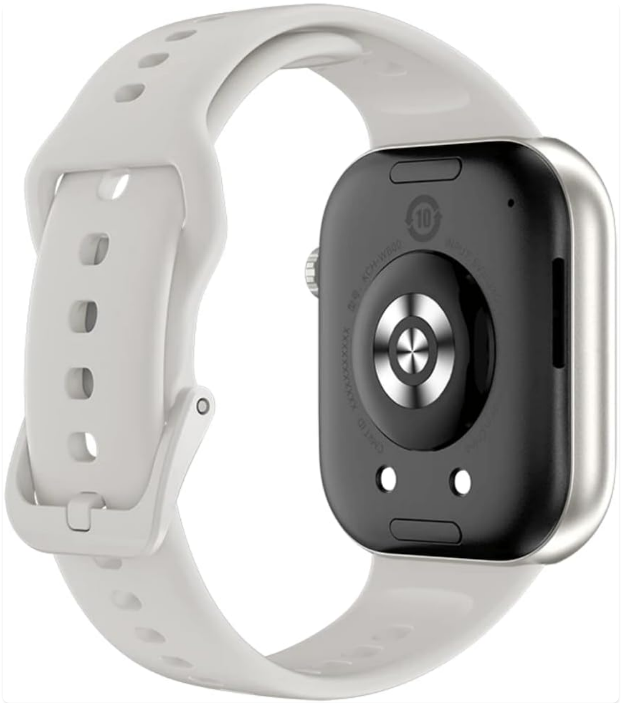
Image 1.1: Rear view of the HONOR Choice Watch 2i, highlighting the charging contacts and health sensors.
