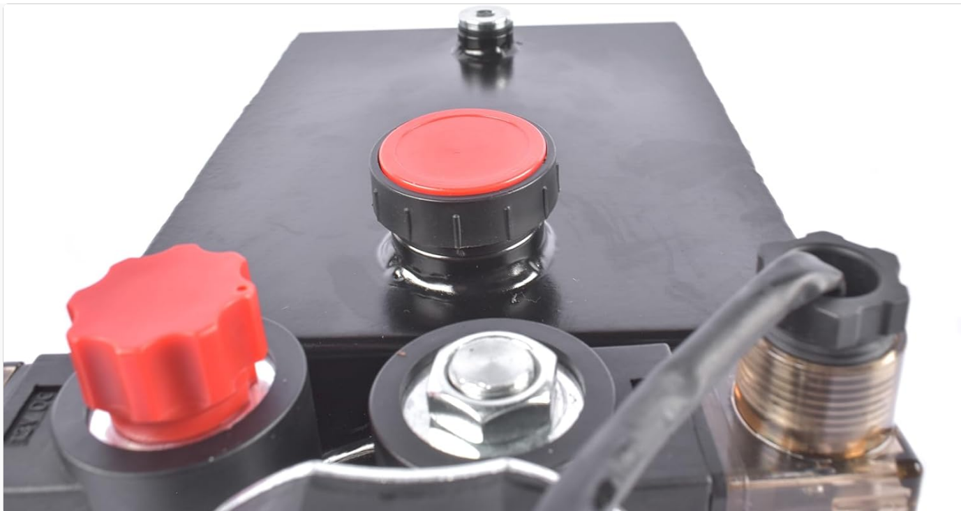
Figure 7: Reservoir cap for fluid checks and refills.
