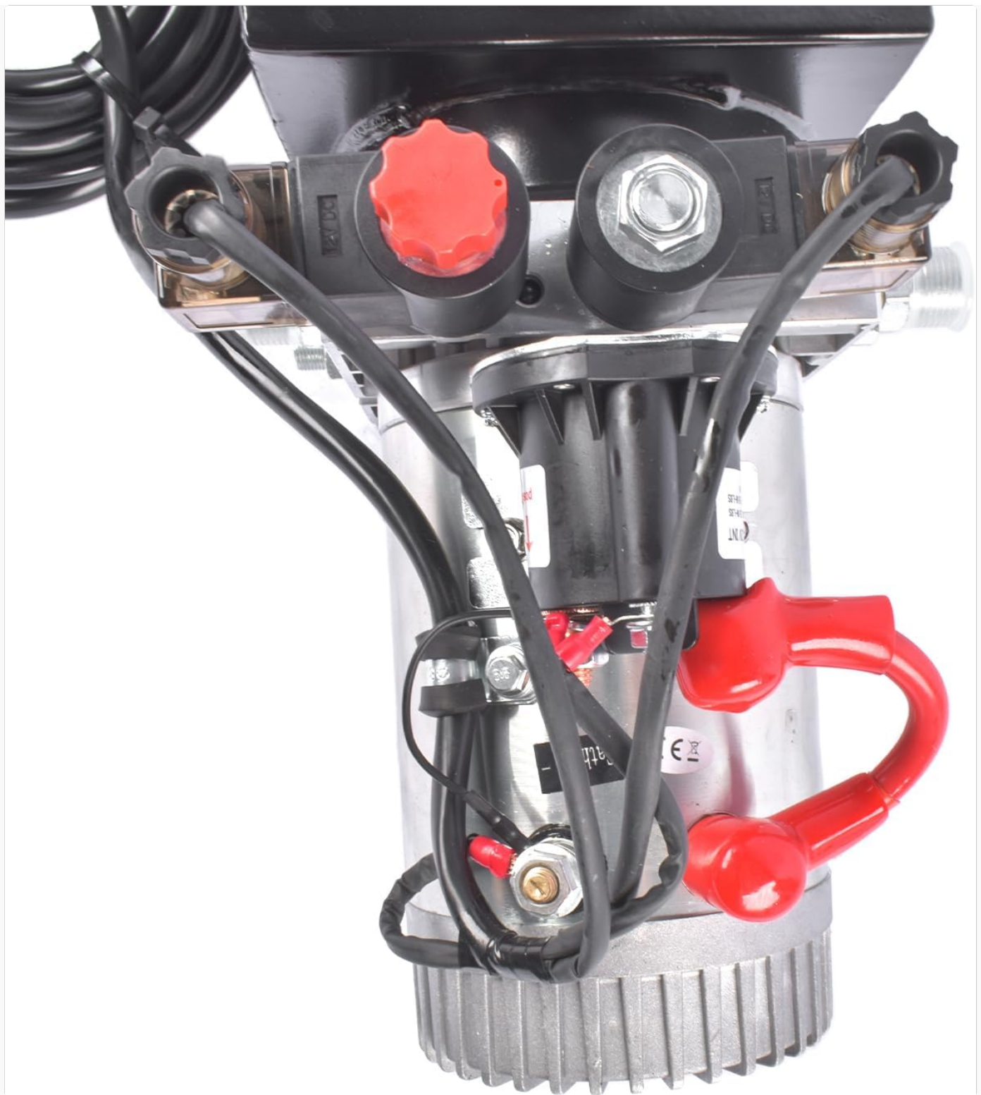
Figure 4: Detail of the electrical wiring connections on the power unit.
