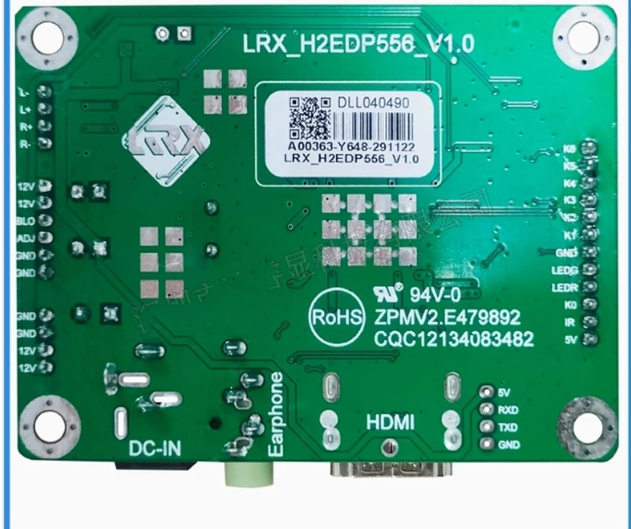
Figure 4: Back view of the EDP driver board. This image shows the reverse side of the board, highlighting important identifiers such as LRX_H2EDP556_V1.0, A00363-Y648-291122, and DLL040490. It also indicates the DC-IN, HDMI, and Earphone ports from this perspective.
