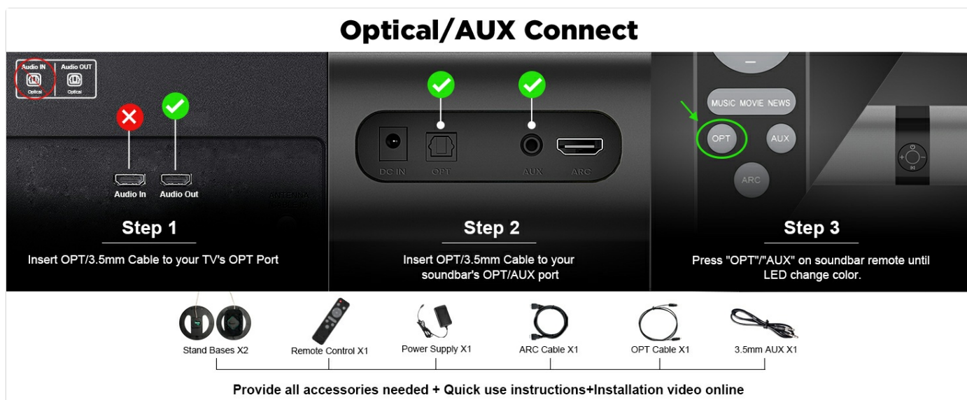
Image: Steps for Optical/AUX connection.
