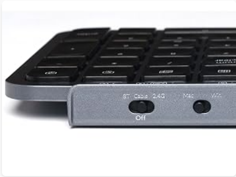
Image: Side profile view of the Keychron B6 Pro keyboard, illustrating its ultra-slim design and the fixed 3.2-degree ergonomic tilt for comfortable typing.
