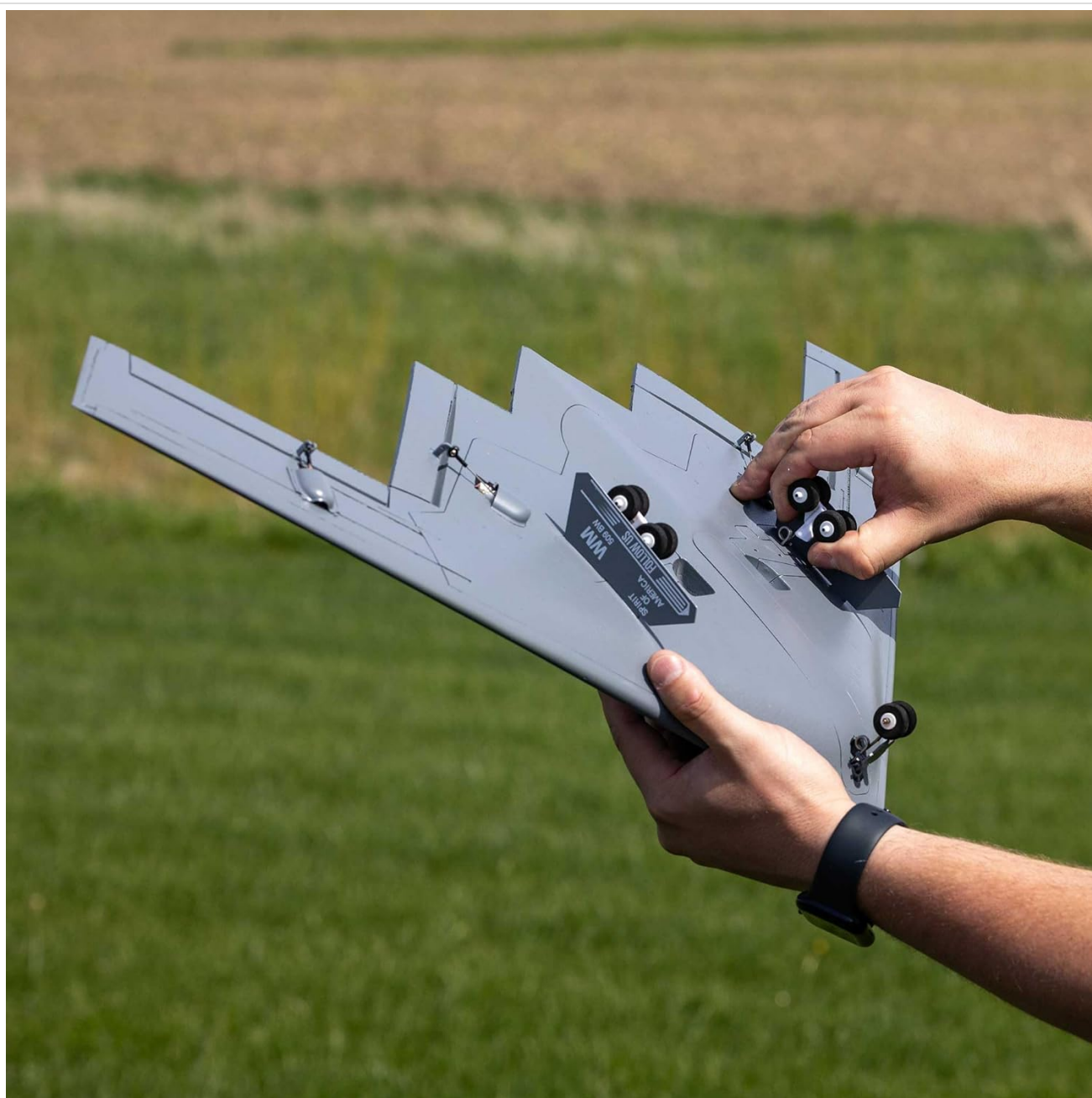
Image: Attaching Optional Landing Gear. A pair of hands is shown attaching the optional fixed landing gear wheels to the underside of the E-flite Micro B-2 Spirit model, demonstrating the assembly process.
