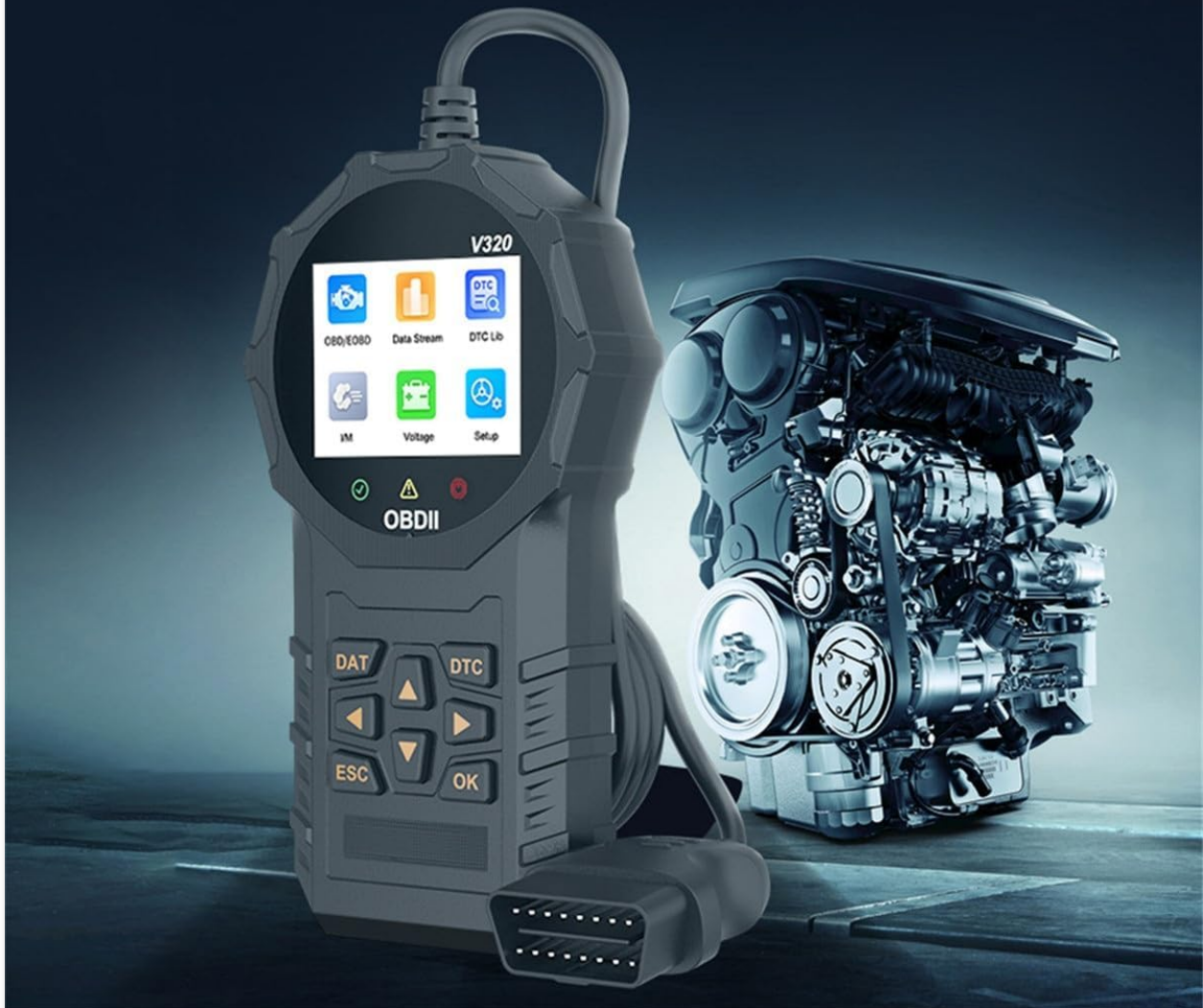
Figure 3.2: XAUCY V320 OBD2 Scanner with labeled parts. This diagram provides a detailed overview of the XAUCY V320 OBD2 Scanner's components. It points out the 2.8-inch color display screen, the 'DAT' button for data stream, the 'DTC' button for reading codes, the directional keys for navigation, the 'ESC' button to return, the 'OK' button to confirm, and the OBD interface connector. It also indicates the power status and fault detection indicators.
