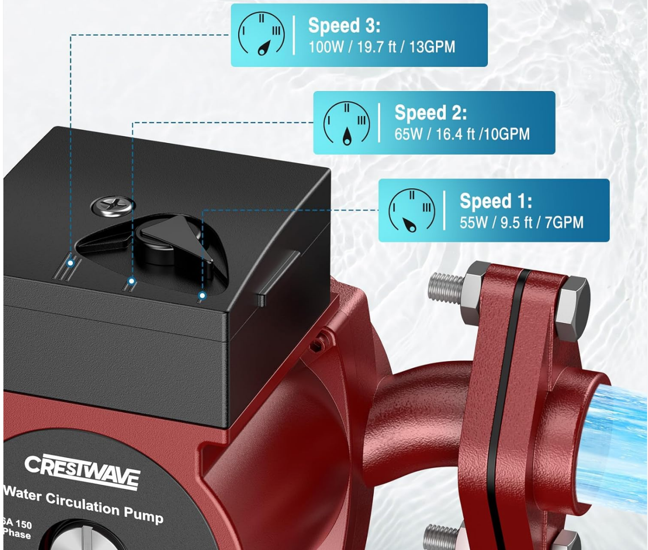
Image 3.1: The pump features three adjustable speed settings for optimized performance. Speed 1: 55W/9.5ft/7GPM, Speed 2: 65W/16.4ft/10GPM, Speed 3: 100W/19.7ft/13GPM.
