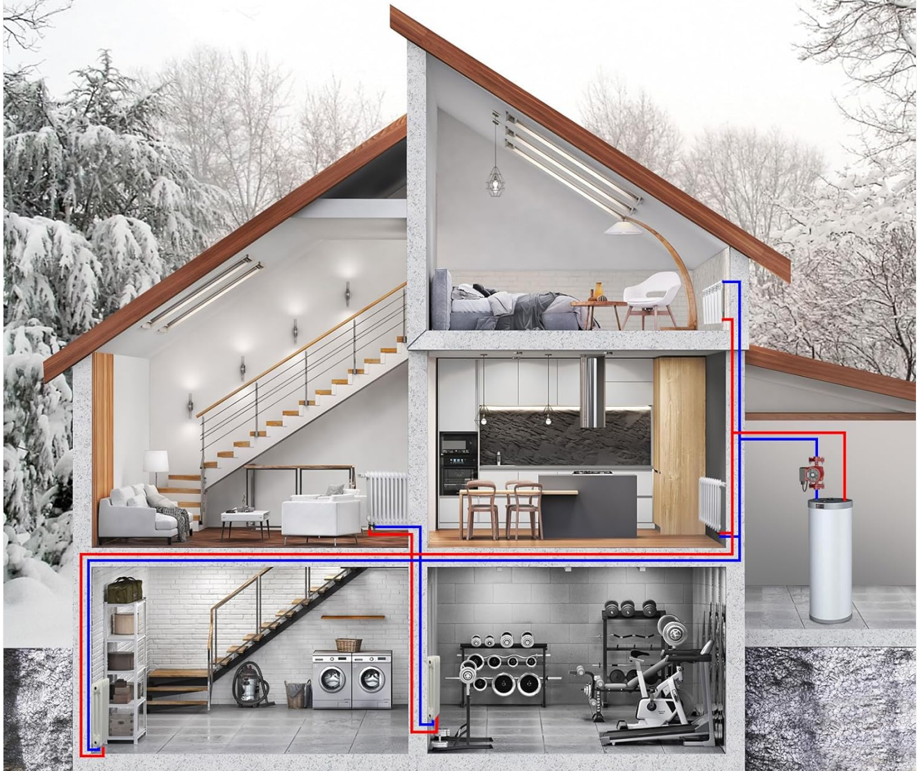
Image 5.1: Illustration of a typical domestic hot water recirculating system within a house, showing how the pump integrates to provide instant hot water at various faucets.
