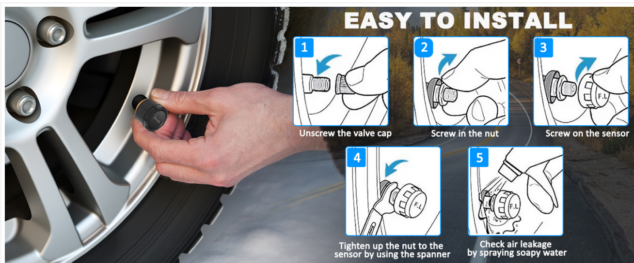
Figure 3: Detailed steps for installing the external tire pressure sensors.
