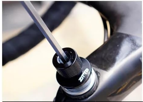
Step2 Install the adapter nut
