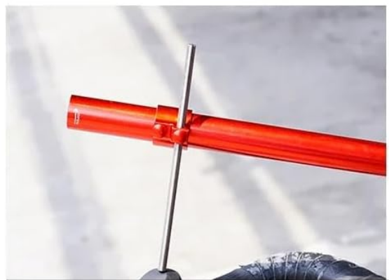
Step4 Adjust measure lever height
