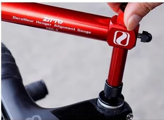
Step3 Install hanger Alignment Gauge
