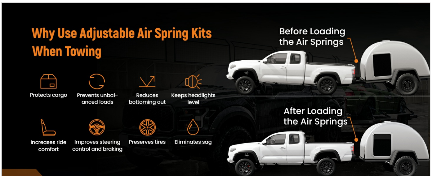
Image 4.1: Load Leveling Comparison. This diagram illustrates the difference in vehicle stance before and after loading with and without the air suspension kit, highlighting how the air springs maintain a level ride height.
