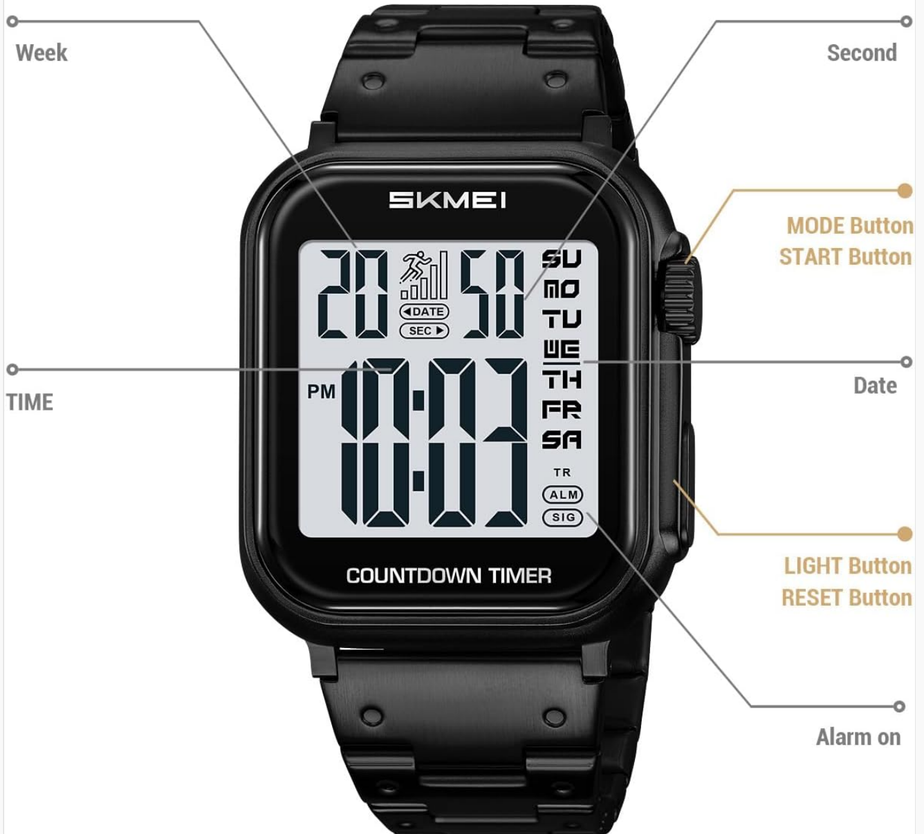
Image: Diagram illustrating the watch's buttons and their functions: MODE/START button, LIGHT/RESET button, and display areas for time, date, week, and alarm status.
