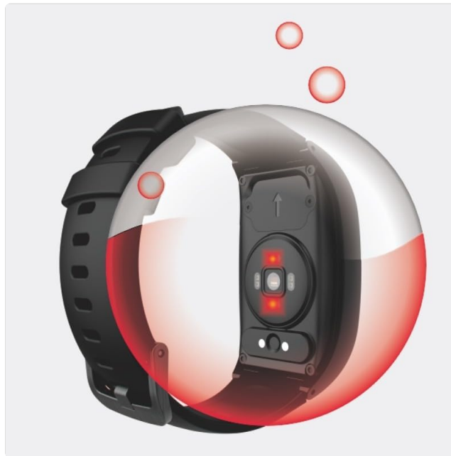
Figure 3.2: Rear view of the L16PRO Smart Watch, highlighting the PPG, SpO2, and temperature sensors.
