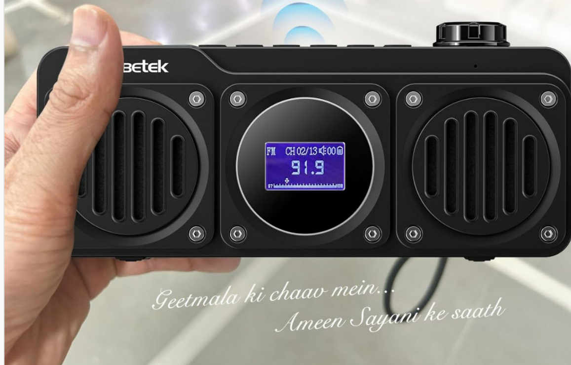
Figure 5.1: FM Radio Display. This image shows the speaker's LCD screen displaying an FM frequency, indicating it is in radio mode.
