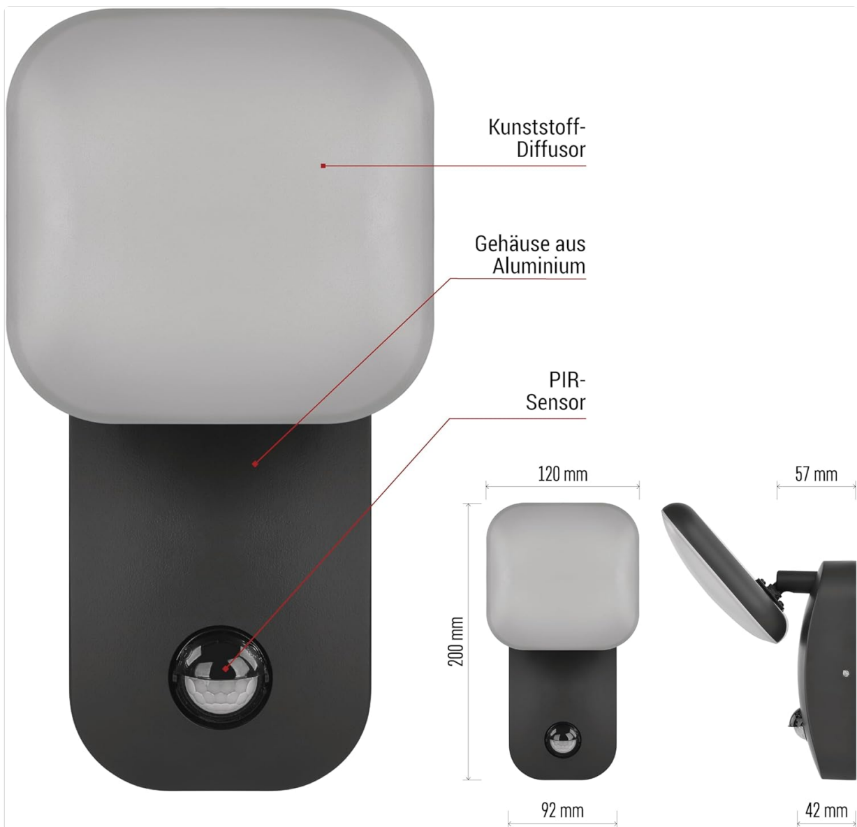
Image: Detailed view of the EMOS NIKA LED Outdoor Wall Light showing its plastic diffuser, aluminum housing, PIR sensor, and dimensions (120mm width, 200mm height, 57mm depth).
