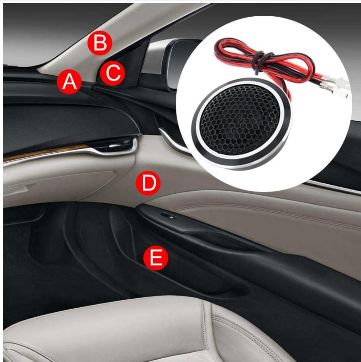
Image: Car Interior Installation Points. This image illustrates various suitable locations for tweeter installation within a car's cabin, such as the A-pillar (A, B, C) and door panels (D, E).
