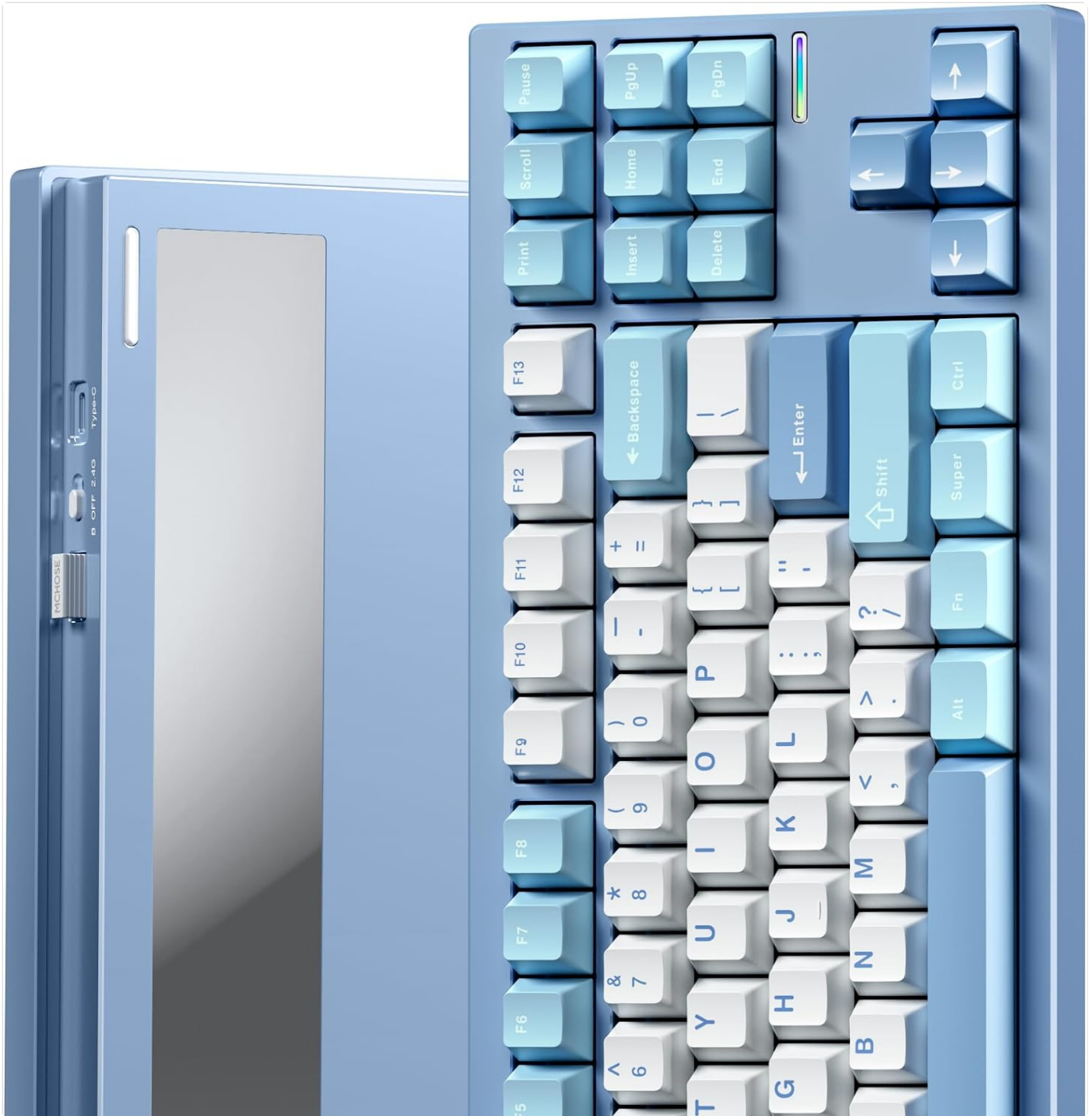
Figure 4.1: Side view of the keyboard, indicating the location of the connectivity mode switch.
