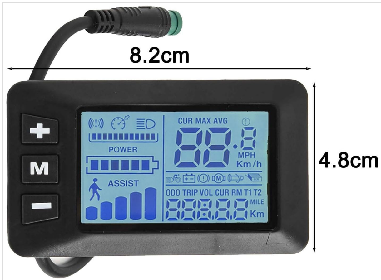
Image 5.1: The GD01 display showing its physical dimensions, 8.2 cm in length and 4.8 cm in height, for reference during installation.
