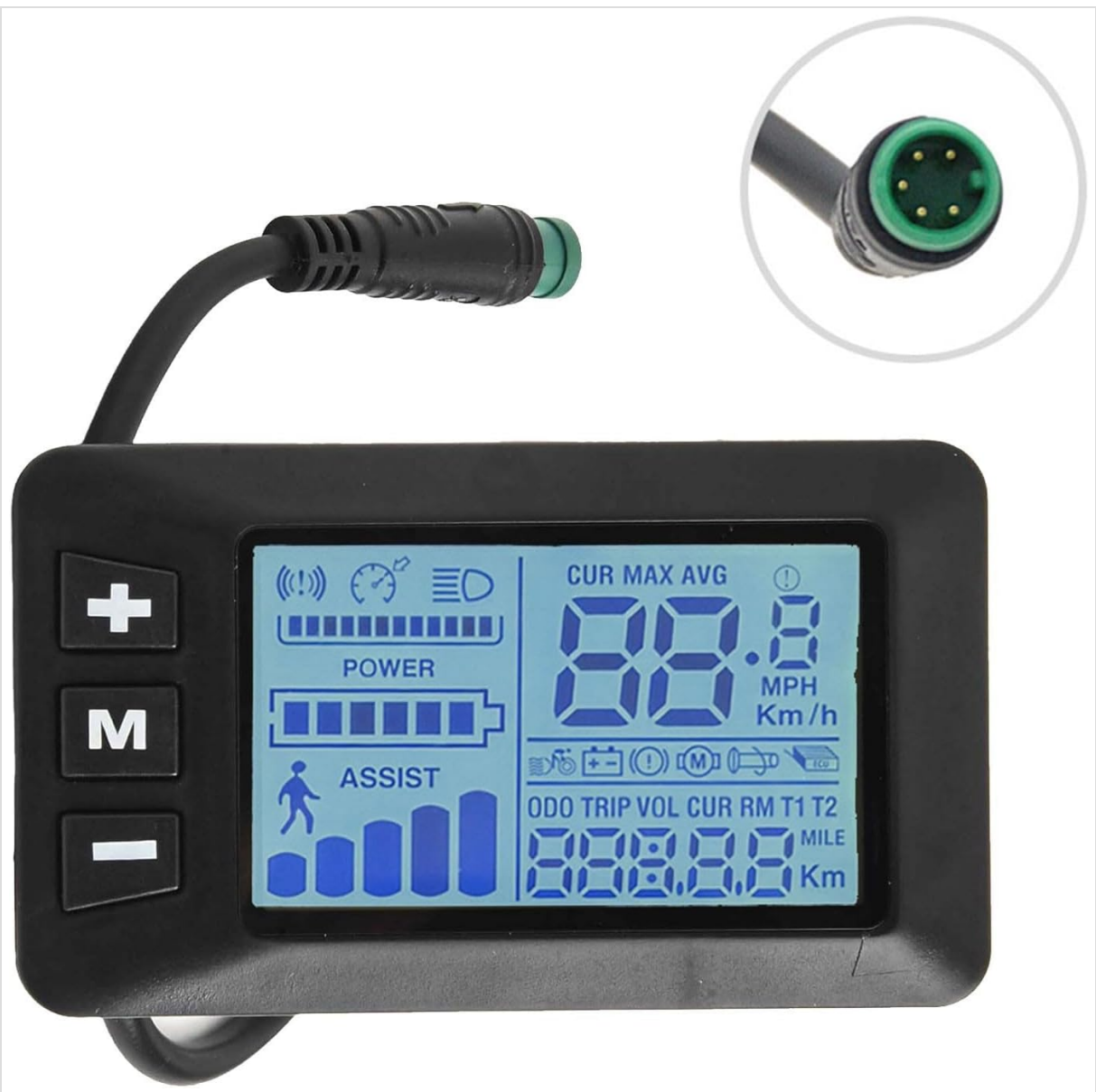
Image 4.2: Detailed view of the GD01 display screen, illustrating the information presented during operation, including current speed, battery status, pedal assist level, and trip data.
