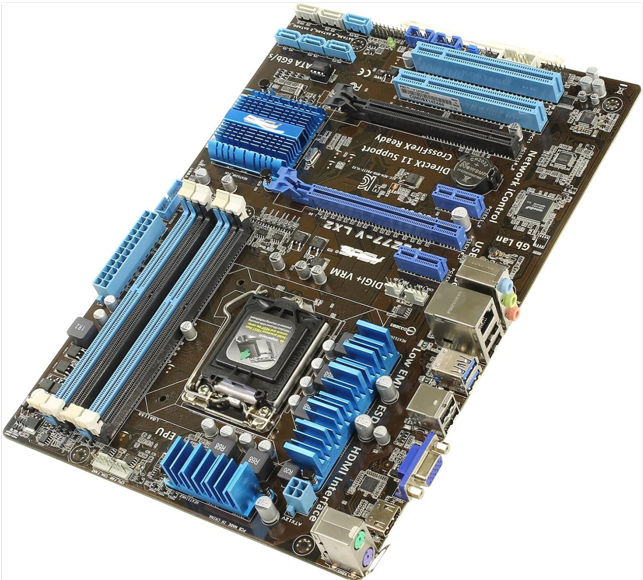
Figure 2.2: Angled view of the ASUS P8Z77-V LX2 Motherboard. This perspective provides a clearer view of the rear I/O panel, including USB ports, video outputs, and audio jacks, as well as the overall layout of components on the board.
