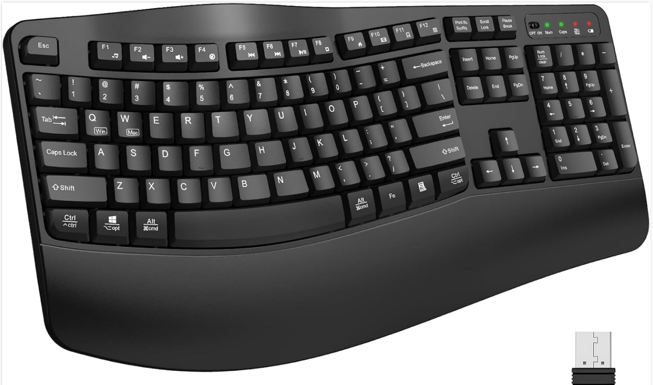
Image 1.1: The EDJO K399 Ergonomic Wireless Keyboard, showcasing its curved design and integrated wrist rest.
