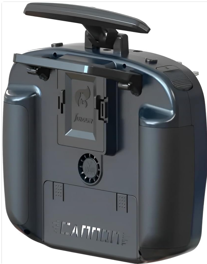
Figure 3.3: Rear view of the Jumper T14, showing the JR module bay, cooling fan, and battery compartment cover.
