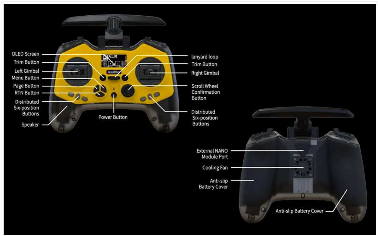
Figure 2.1: Front and Rear View of the Jumper Bumblebee Transmitter with Labeled Components.
