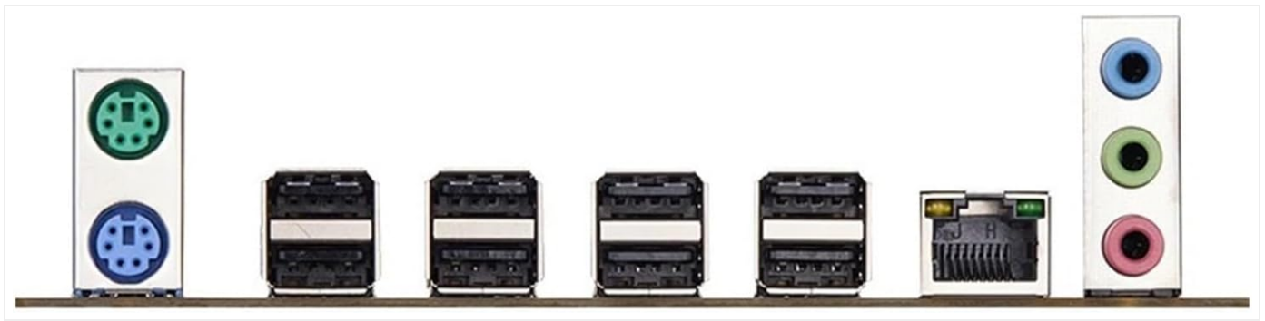
Figure 1.5: Rear I/O panel showing PS/2 ports, USB ports, RJ45 network port, and audio jacks.
