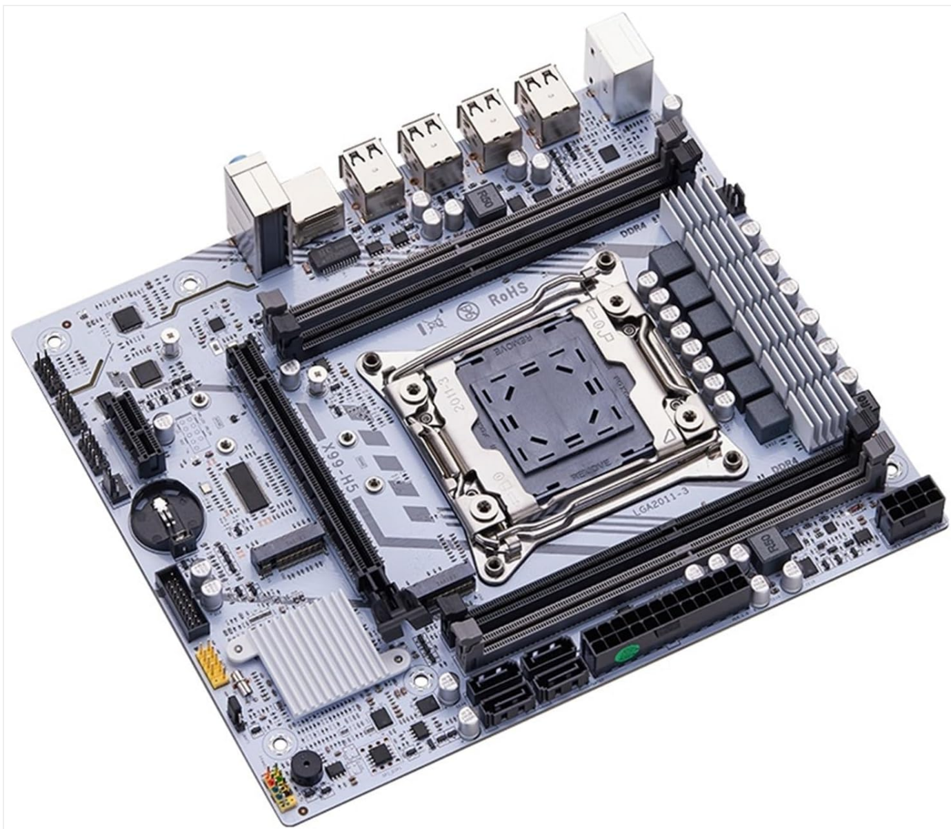
Figure 1.2: Angled view of the NNHUNYI X99 H5 Motherboard, showcasing its layout and cooling armor.
