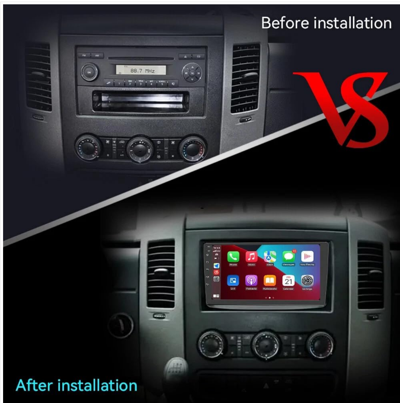
Image 2.1: A visual comparison showing the original car radio setup (top) versus the Surakey Car Stereo Radio installed (bottom) in a Mercedes Benz Sprinter dashboard.
