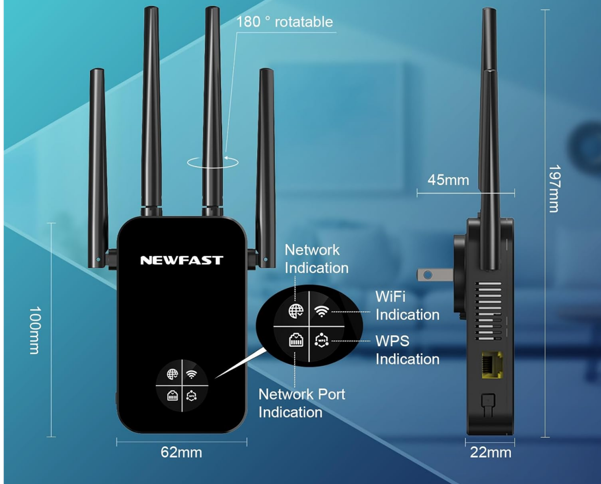
Figure 3.1: Front and side view of the NEWFAST RE523 WiFi Extender, illustrating its dimensions (100mm height, 62mm width, 22mm depth) and the location of the Network Indication, WiFi Indication, WPS Indication, and Network Port Indication lights. The antennas are 180° rotatable.
