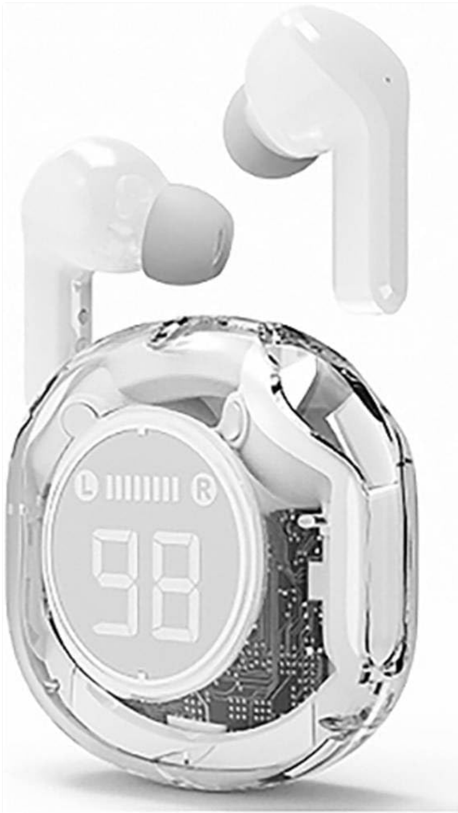
Figure 3.1: The Gembird TWST-01-W Transparent Bluetooth Earbuds shown within their charging case. The case features a clear design, revealing the internal components and an LCD display indicating battery levels for both earbuds (L and R) and the case itself.
