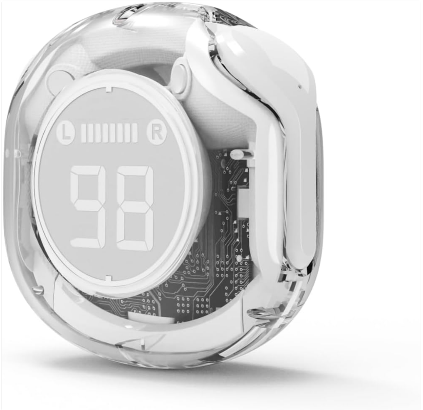
Figure 4.1: Side view of the Gembird TWST-01-W charging case, highlighting its transparent construction and the integrated LCD battery display. The charging port is typically located at the bottom or rear of the case.
