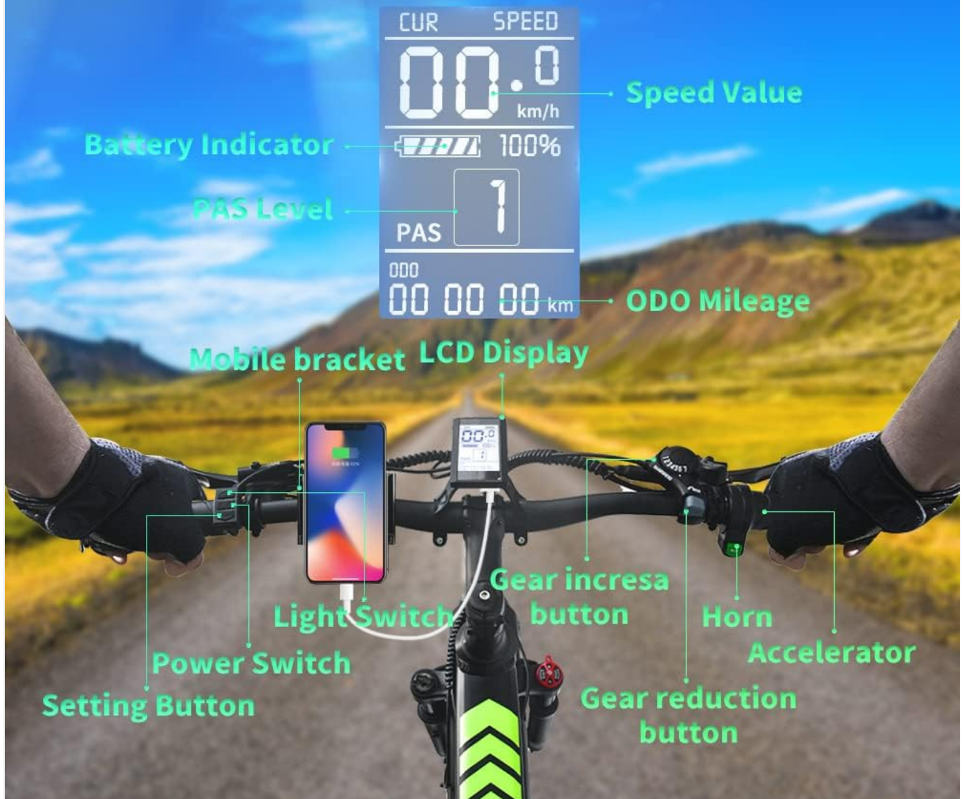
Figure 4: The intelligent LCD display provides real-time information such as current speed, battery indicator, PAS level, and total mileage.
