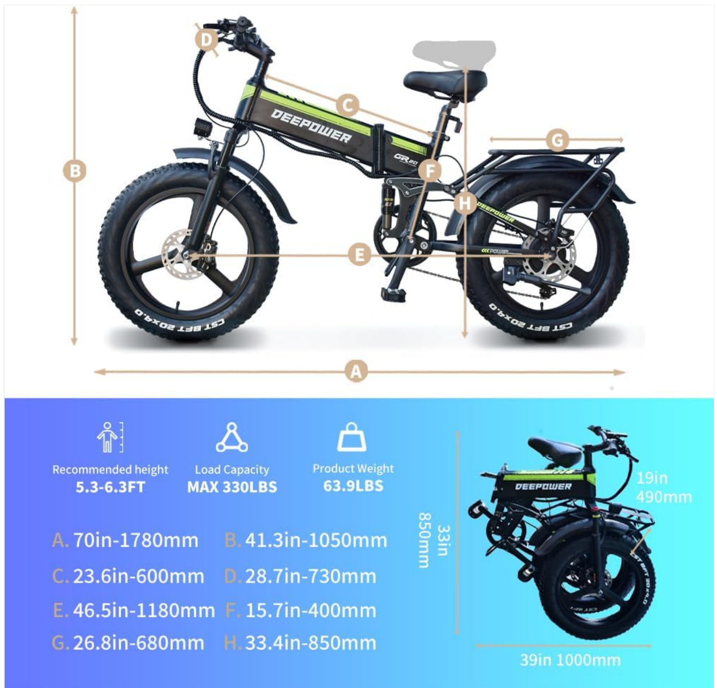
Figure 12: Detailed dimensions and load capacity information for the DEEPOWER H20pro, including recommended height and product weight.
