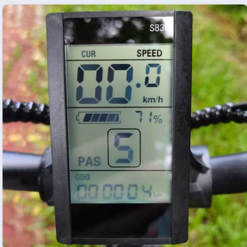
Figure 4: The intelligent LCD display provides real-time information such as current speed, battery indicator, PAS level, and total mileage.
