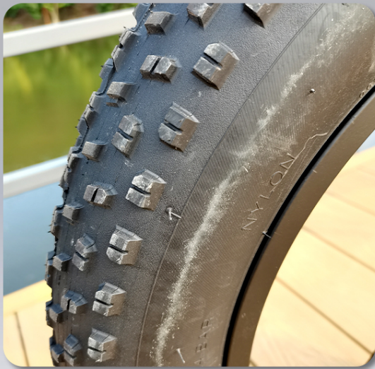
Figure 9: Detail of the 20" x 4.0" off-road fat tire, designed for excellent traction and support across diverse terrains.
