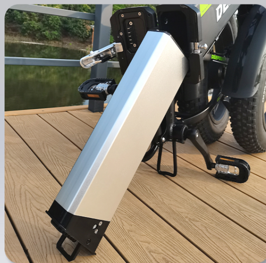
Figure 3: Demonstrating the removal of the integrated battery for charging or storage.
