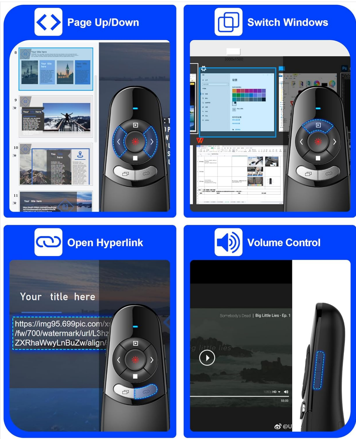
Image: Diagram illustrating the various functions of the presentation clicker buttons, including page navigation, window switching, hyperlink, and volume control.
