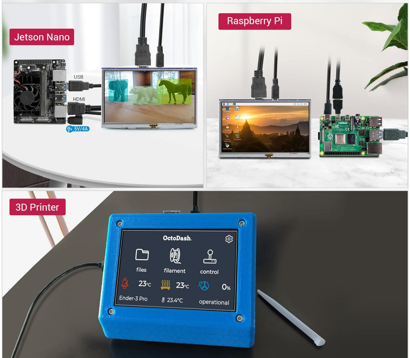
Image: The ELECROW monitors demonstrating compatibility with various applications, including connection to a Jetson Nano, a Raspberry Pi setup, and integration as a 3D printer interface.
