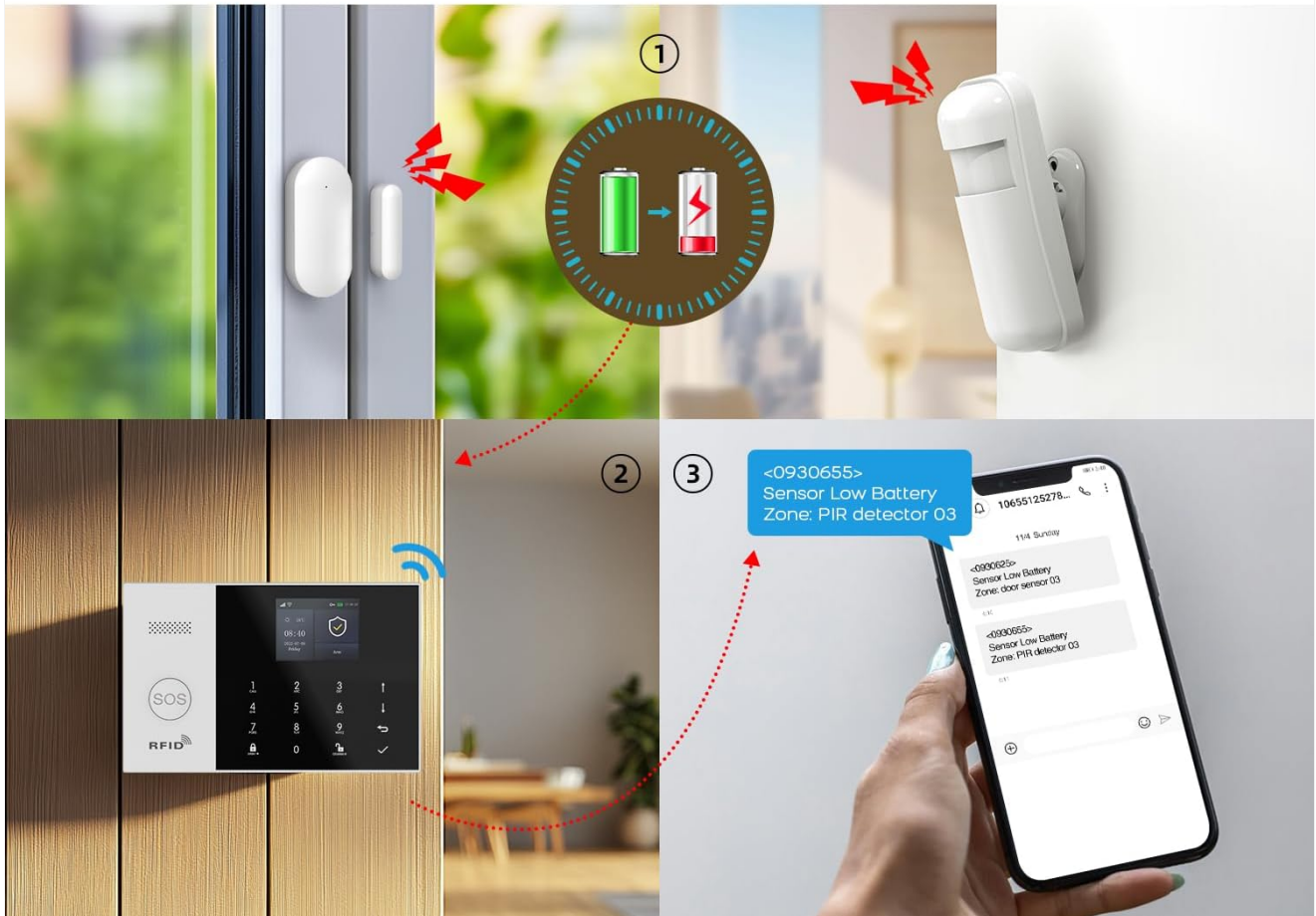
Image 4.1: Illustration of a wireless sensor indicating low battery, which then sends a signal to the host, and the host pushes a notification to the user's app.
