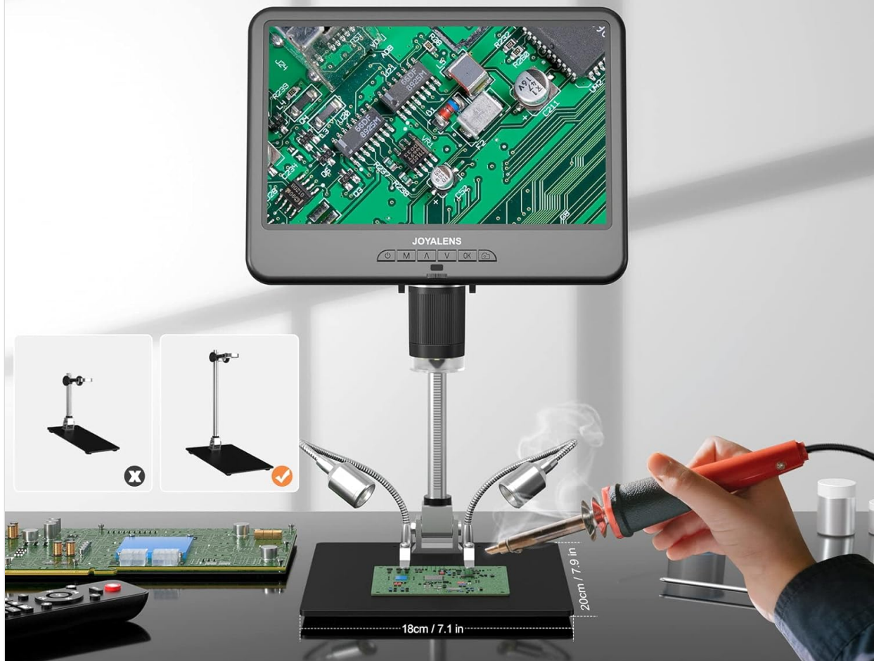
Figure 3.2: The JL210 Digital Microscope set up on its large metal base, providing a stable and spacious workbench for soldering and electronic repair tasks. The image shows the microscope positioned over a circuit board with a soldering iron in use.
