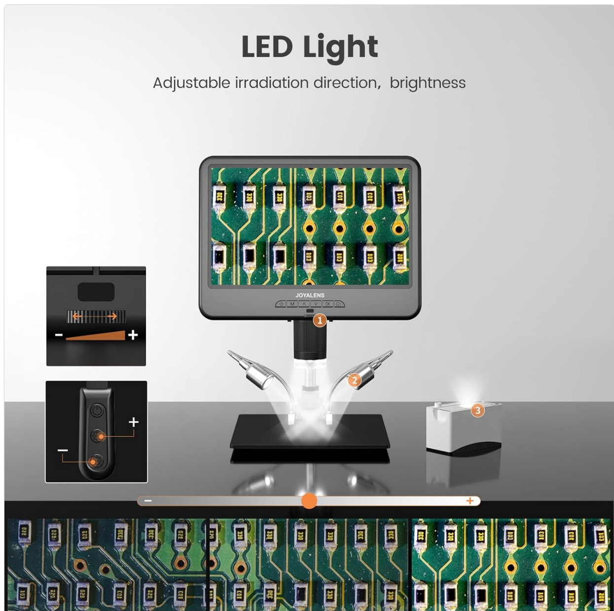
Figure 4.1: An illustration detailing the LED light adjustment features of the JL210 Digital Microscope, showing controls for
