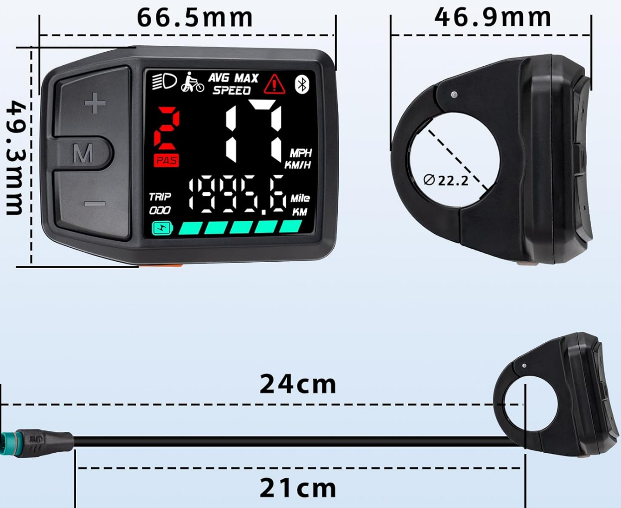
Image 3.2: Technical drawing detailing the physical dimensions of the DZ41 display (66.5mm x 49.3mm) and its handlebar clamp (22.2mm diameter), along with cable lengths (24cm total, 21cm to connector).
