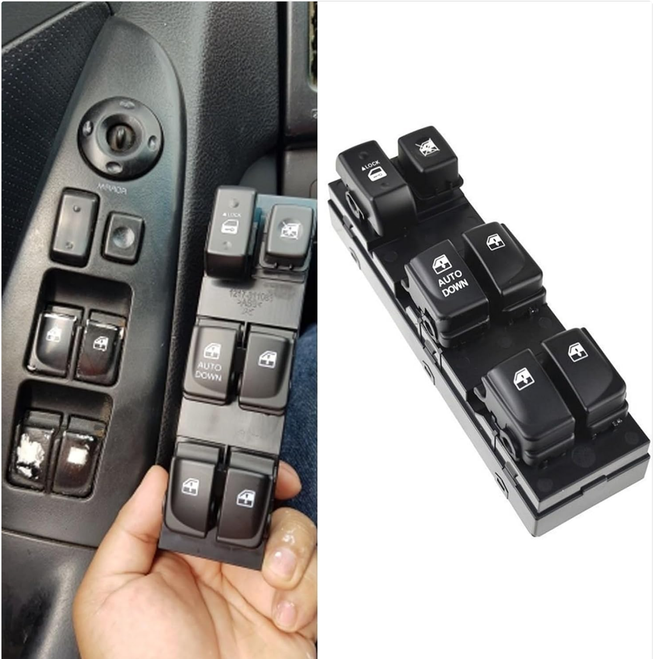
Figure 4.1: Visual comparison of the old switch being removed and the new switch ready for installation, demonstrating the direct fit.
