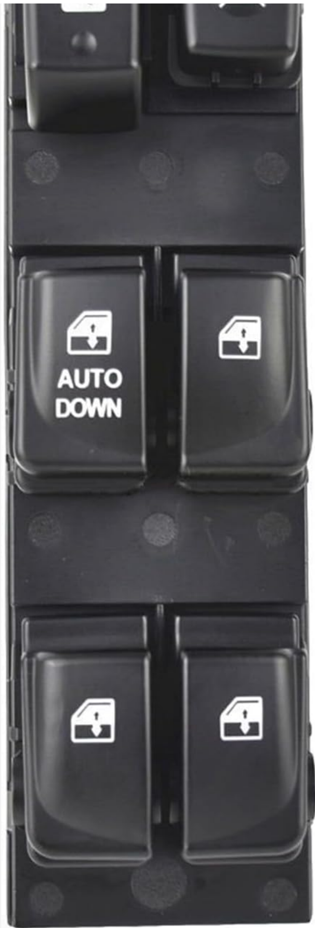
Figure 3.2: Top-down view of the switch, highlighting the layout of the individual window control buttons and the master lock buttons.
