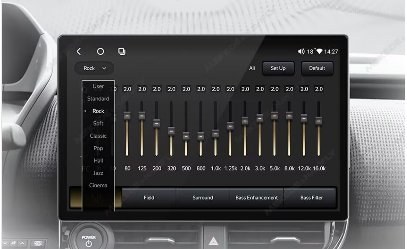
Image: DSP Equalizer Adjustments. This image shows the graphical interface of the DSP equalizer on the car stereo, with sliders for various frequency bands and preset options like Rock, Pop, Jazz, and Cinema.
