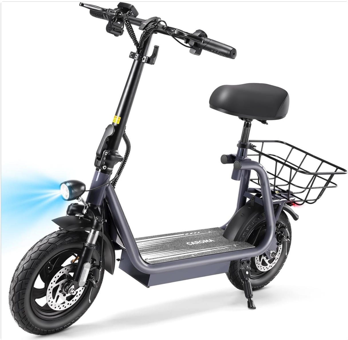
Figure 3.1: The Caroma Peak 819W Electric Scooter Q2, showcasing its overall design, front headlight, adjustable seat, and rear storage basket.
