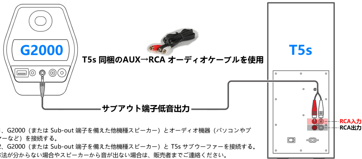
Figure 4: Connection diagram showing how to connect the Edifier T5s Subwoofer to Edifier G2000 speakers using the included AUX to RCA audio cable.
