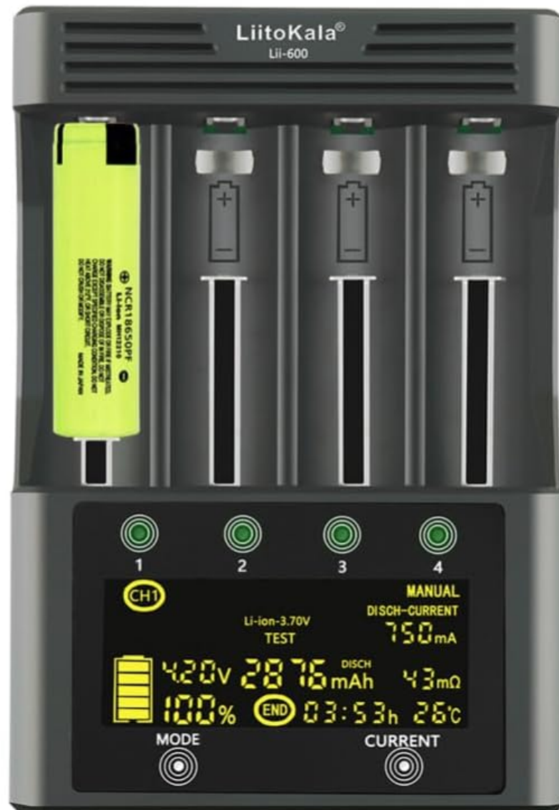
Figure 6.1: Example of a capacity test in progress.
