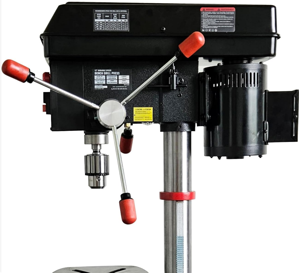
Image 2.2: View of the powerful 6-pole motor, designed for low speed and high torque applications.
