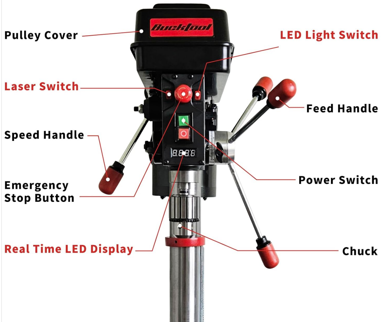
Image 2.1: Labeled components of the BUCKTOOL 12-inch Benchtop Drill Press. Key components include the Pulleys Cover, LED Light Switch, Laser Switch, Speed Handle, Emergency Stop Button, Real Time LED Display, Chuck, Feed Handle, and Power Switch.
