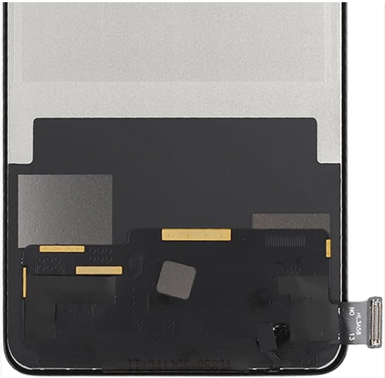
Figure 4.2: Rear view of the replacement TFT LCD display, highlighting connection areas.
