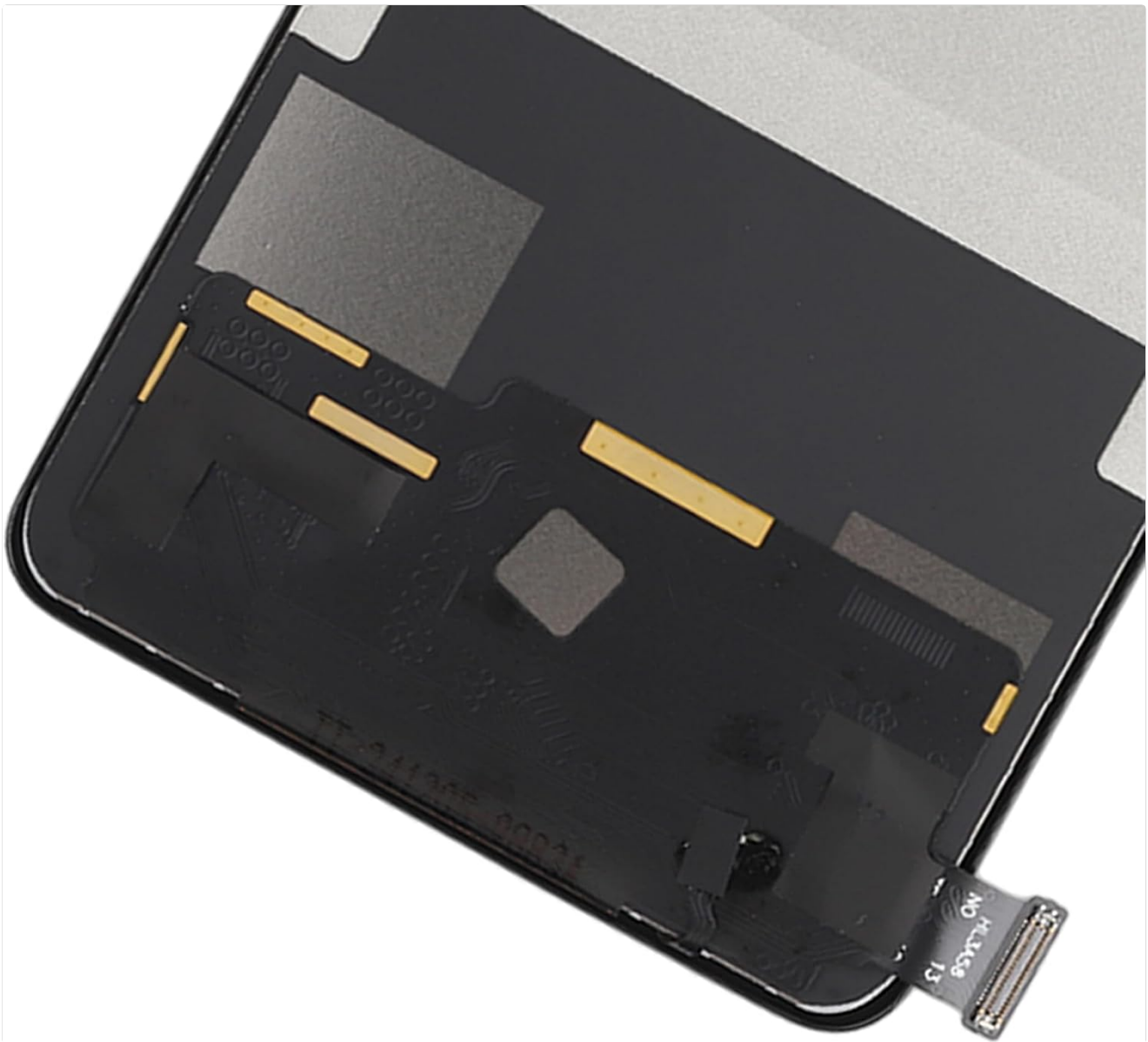
Figure 4.3: Detailed view of the flex cable, a critical component for display functionality.
