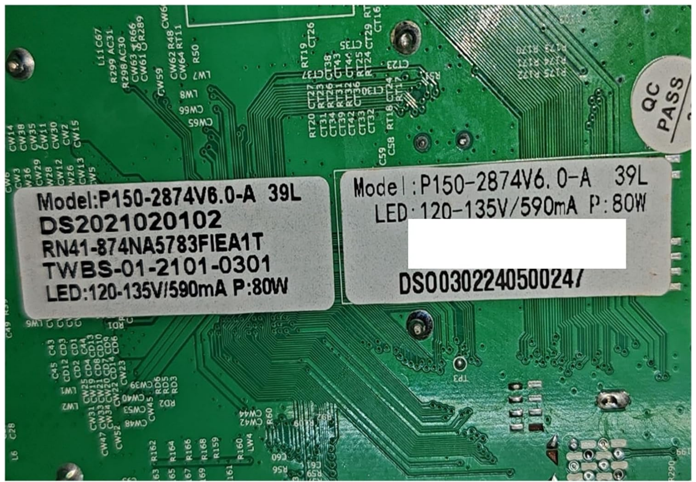
Figure 4.1: Example label for P150-2874V6.0-A 39L variant, showing LED: 120-135V/590mA, P: 80W.
