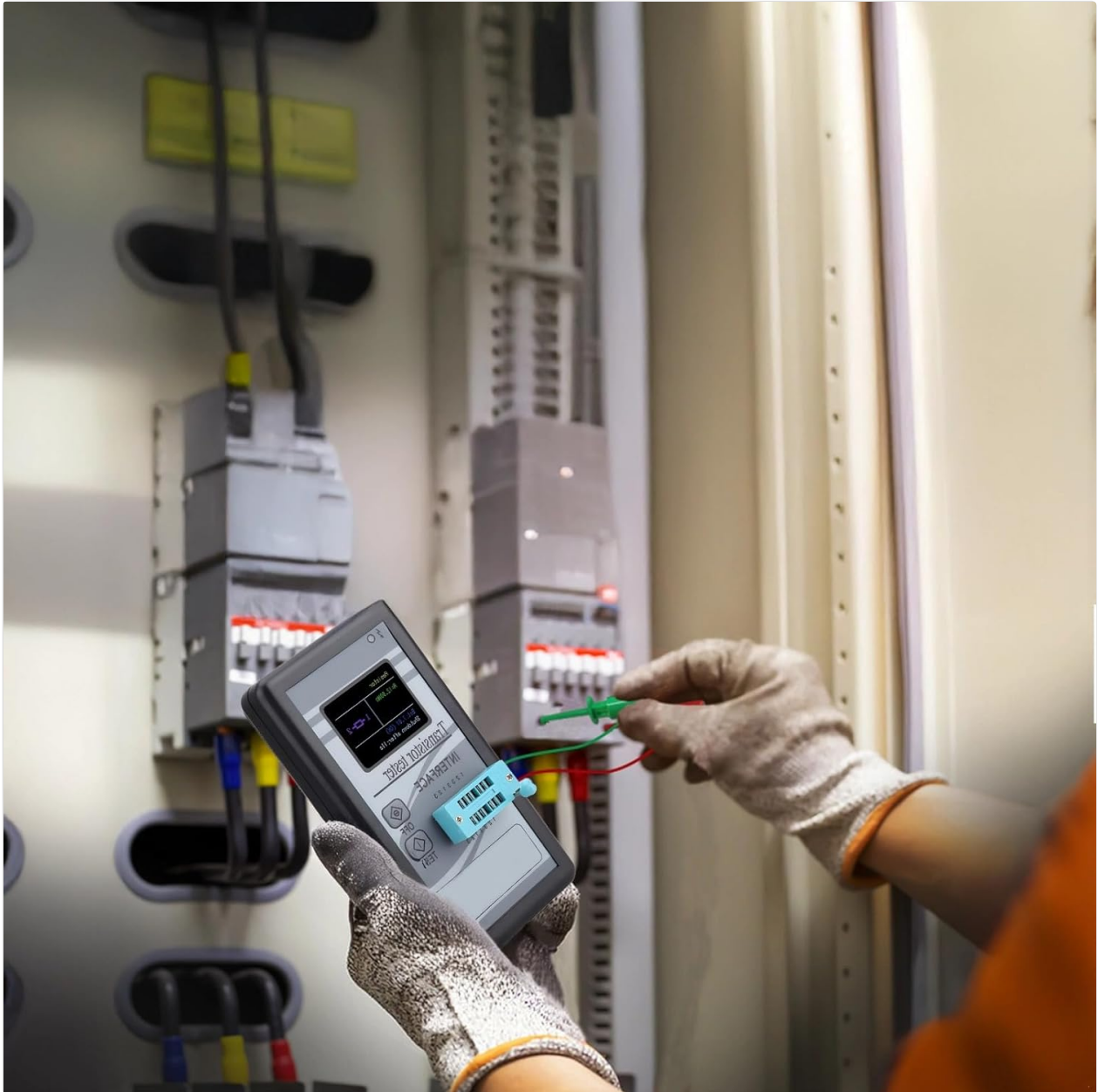
User operating the M328 Transistor and Component Tester to test an electronic component.
